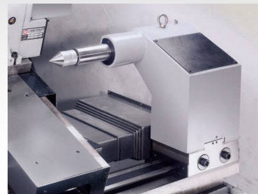
尾座 Tail Stock 可程式頂針行程100mm Programmable quill with stroke 100mm and MT4 taper.
